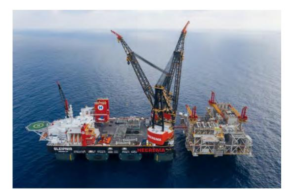
The Sleipnir is designed for worldwide offshore heavy lifting. It is equipped with two cranes of 10,000 metric tonnes lifting capacity each and a reinforced deck area of 220 meters in length and 102 meters in width, which make it the largest crane vessel in the world.
