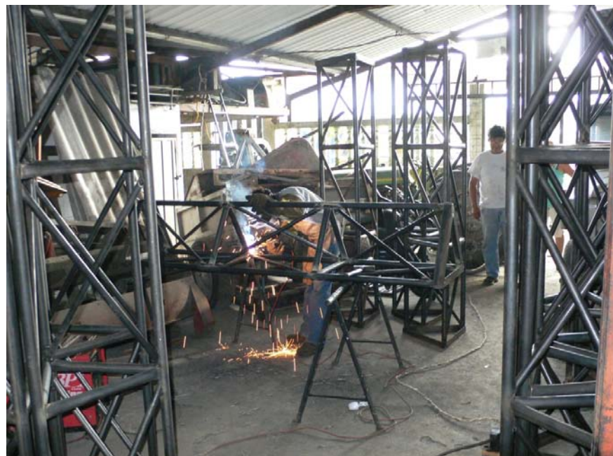
Construction of towers and supports for the photovoltaic modules
